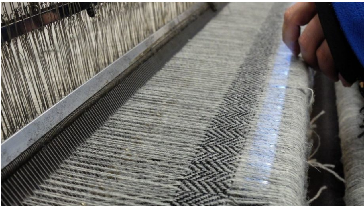
Fig. 1. Weaver setting up the loom to start weaving a new length of Harris Tweed in a black and grey herringbone pattern, 2017. © Joana Nascimento
